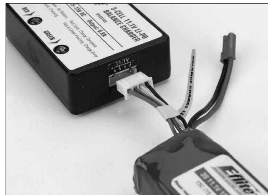
When the battery is properly connected and charging normally, the red and green LED indicators will glow solid. Once the battery has been fully charged, the green LED will go out, leaving just the red LED glowing solid. The battery can now be removed from the charger and installed into the Blade SR for flight.
