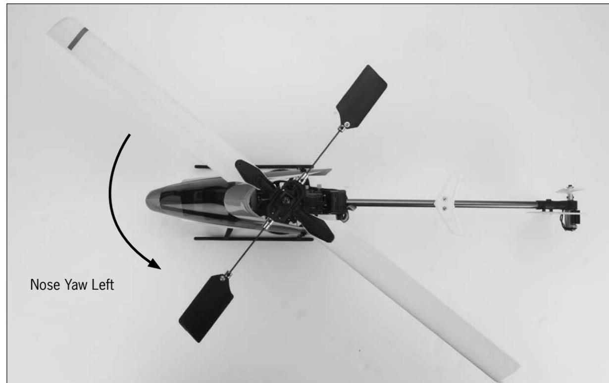
Moving the stick to the right will turn (yaw) the nose of the helicopter to the right about the axis of the main shaft. This is accomplished by increasing the speed of the tail rotor blade.
