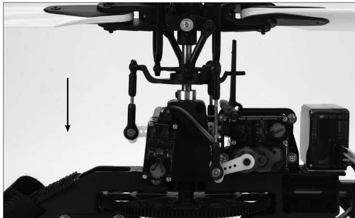
With the stick pulled back down, the swashplate should raise, decreasing the pitch of the main blades.
