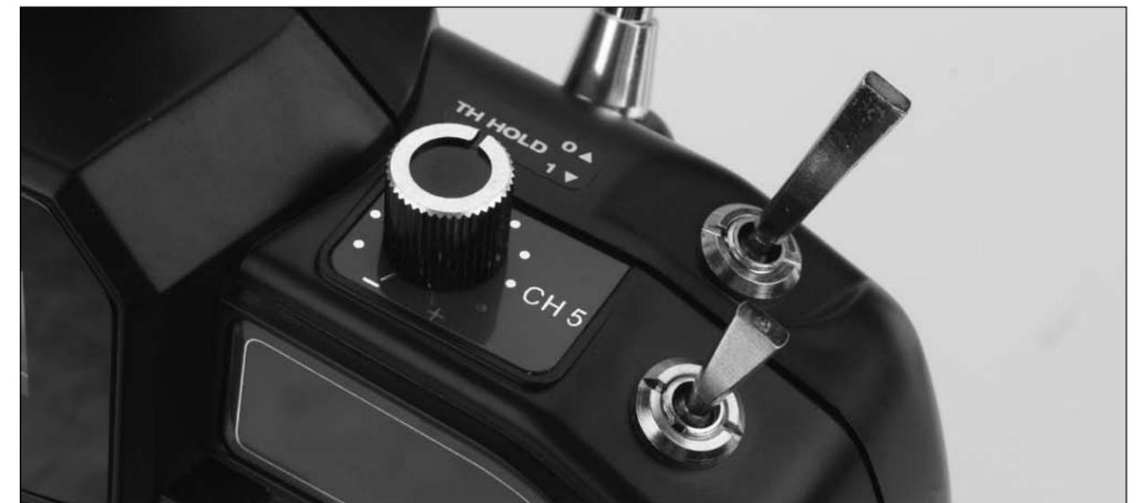
When the throttle hold switch is toggled toward the front of the transmitter (position 1), throttle hold will be on (activated). Toggling the throttle hold switch to the on position also allows you to safely power down the 2-in-1/motors any time the helicopter is not flying. This allows you to safely handle the helicopter, while the 2-in-1 unit is still armed, regardless of the throttle/collective stick and flight mode switch positions.
