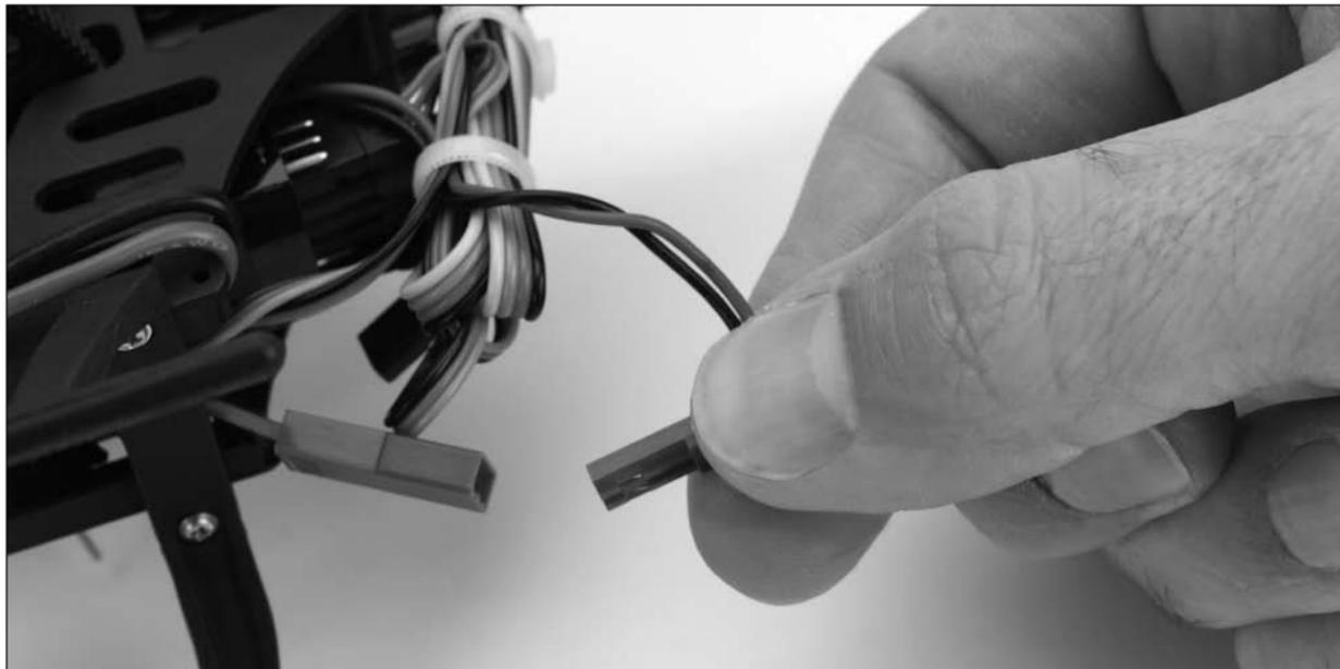
Turn the transmitter on first and lower the throttle stick and trim completely. Then, plug the battery into the battery lead of the 2-in-1 unit.
