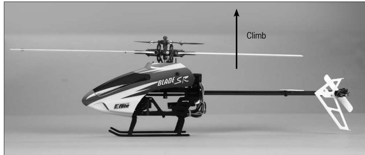
Decreasing the speed and pitch of the main rotor blades by lowering the left-hand stick will cause the model to descend.
