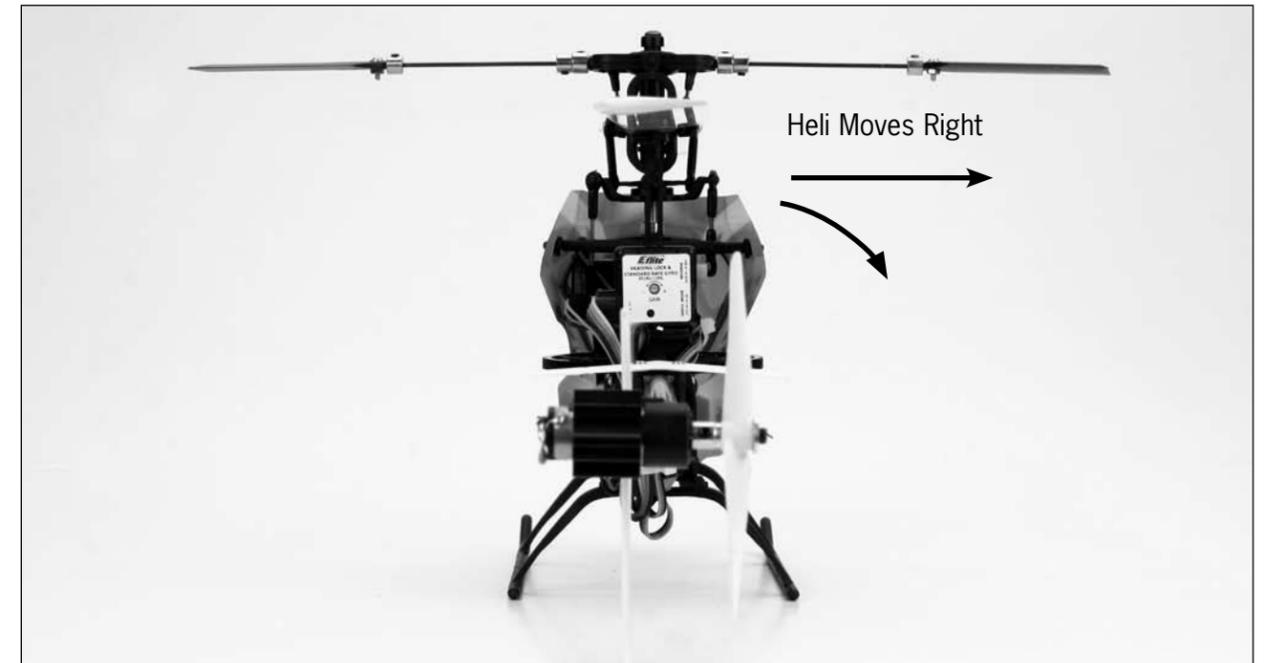
Use the aileron trim to help keep the helicopter from drifting left or right when in hover with no aileron stick input. For example, if the helicopter drifts to the right when in hover, add left aileron trim until the helicopter hovers as level as possible with no drifting to the right.
